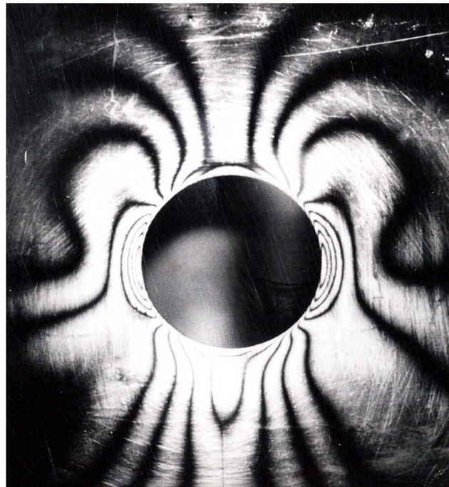
FIG. 28-A Stress Pattern of Unlined Circular Opening
