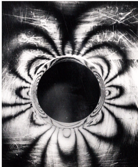
FIG. 31-A Thinnest Lining in Series of Lining Thicknesses, t/R = .177
