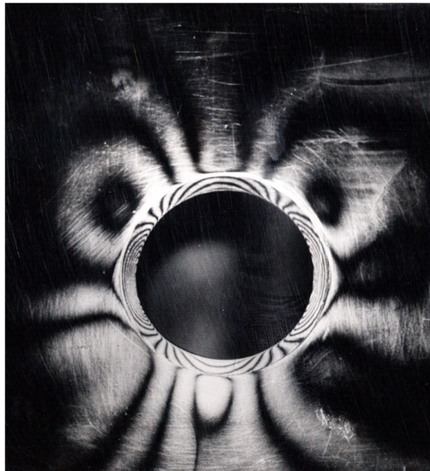
FIG. 30-A Most Rigid Lining, t/R = .177
