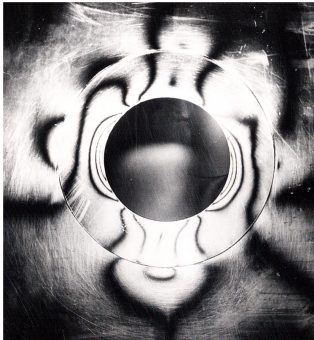
FIG. 35-A Lining Thickness of .904 inches, t/R = .708
