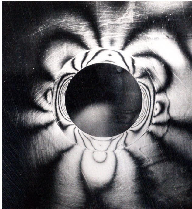
FIG. 33-A Lining Thickness of .452 inches, t/R = .354
